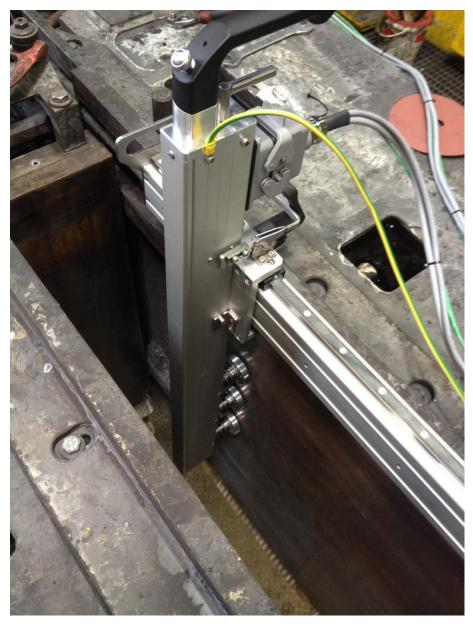
Heating arm of the Thermocouple Checker from Primetals Technologies while measuring functioning of the thermocouples belonging to the broad side of a mold in the installed state. Defective thermocouples and poor contacts can be reliably detected with the system.
