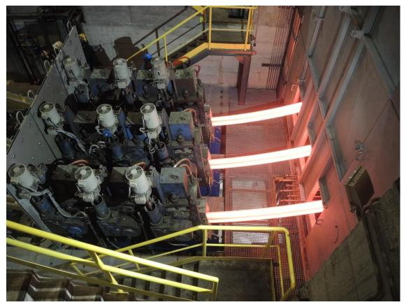
Three-strand continuous billet caster from Primetals Technologies at the Bolzano plant site of Italian steel producer Acciaierie Valbruna S.p.A.
