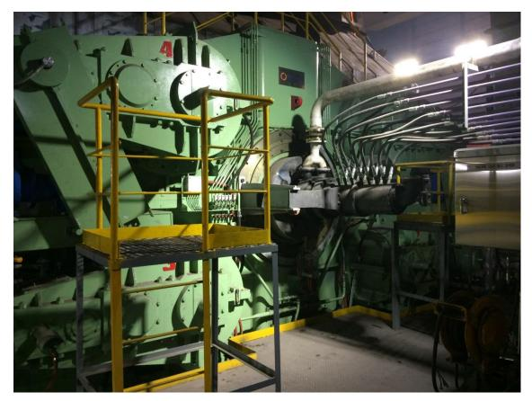
Tilting drive from Primetals Technologies on converter no. 1 in Posco's steel works no.1 in Gwangyang, Korea.
