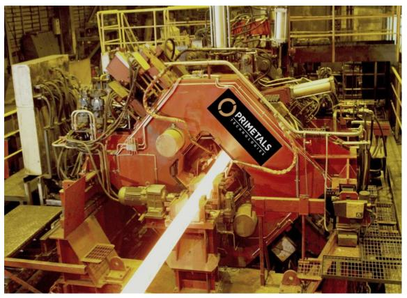
ERT-EBROS billet welding system from Primetals Technologies. A similar system will be installed at the Emirati Union Iron & Steel Company LLC (Union Iron & Steel) company.
