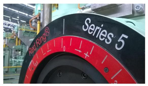
Red Ring generation 5 rolling stand from Primetals Technologies. The new rebar mill of Agha Steel Pvt Ltd (Agha Steel Industries) in Port Qasim near Karachi, Pakistan will be equipped with a total of 16 stands.
