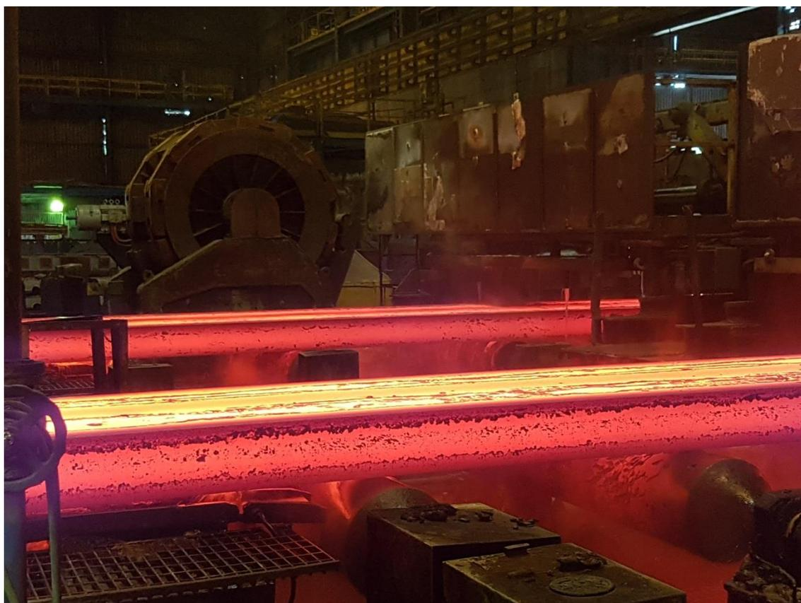
Exit section of a continuous slab caster in the Volta Redonda, Brazil production site of Companhia Siderúrgica Nacional (CSN). Primetals Technologies is revamping three of CSN's continuous casting machines (Photo courtesy CSN).
