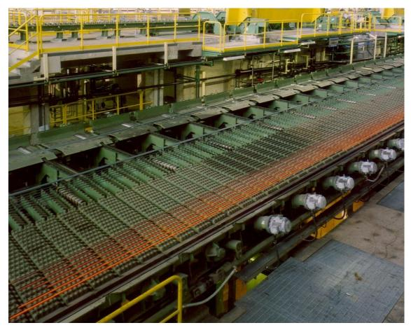
Straight bar on cooling bed. Primetals Technologies will supply upgrade equipment for Charter Steel Cleveland to enter SBQ straight bar market.
