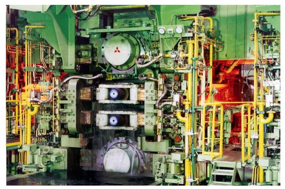
Hot strip mill HSM 1580 of Baoshan Iron & Steel Group Co. Ltd (Baosteel) in Shanghai, China. Primetals Technologies will equip the mill with the technology package "Dynamic Width Control". The aim is to improve the width performance of HSM 1580 and thus reduce the amount of waste material.
