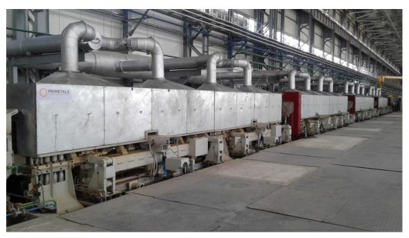
idRHa+ inline rail head-hardening system from Primetals Technologies at the ARBZ rolling mill in Aktobe, Kazakhstan.
