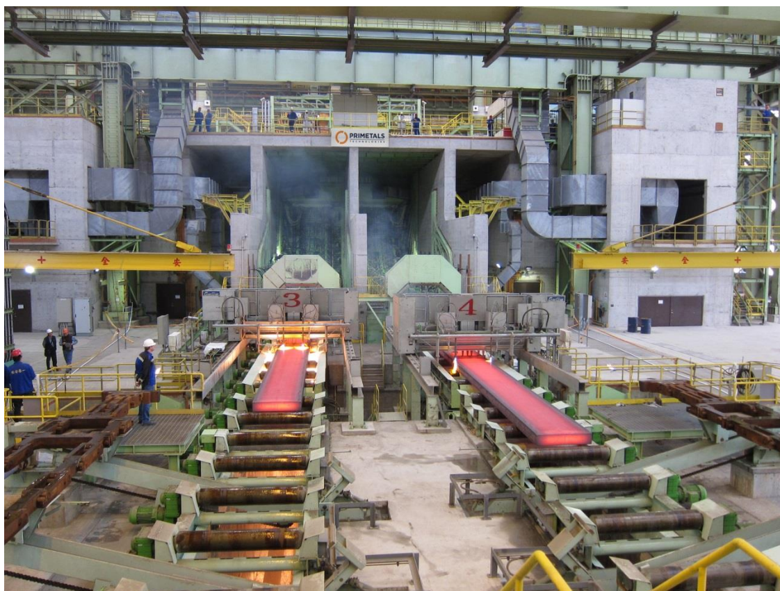
Twin-strand continuous slab caster from Primetals Technologies
