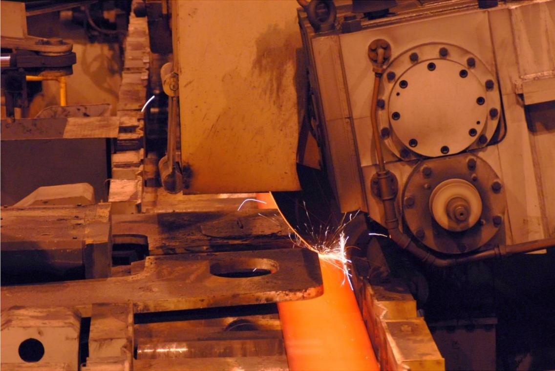
Abrasive-type sawing unit for quality flats from Primetals Technologies. A comparable system will be installed in the bar rolling mill of Çemtaş in Bursa, Turkey.
