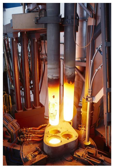
Ladle heating station from Primetals Technologies.
