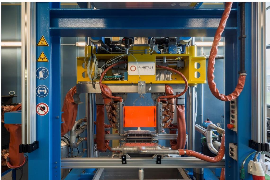
Glühsimulator Multipas (Multi purpose annealing simulator) von Primetals Technologies.
