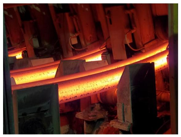
Primetals Technologies modified a continuous caster at Gerdau Cartersville, Georgia in the USA. The project gives the capability to produce an additional beam blank format.
