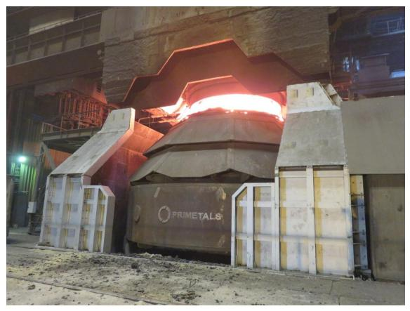
LD (BOF) converter installed by Primetals Technologies at the Dąbrowa Górnicza steel works for ArcelorMittal Poland S.A.
