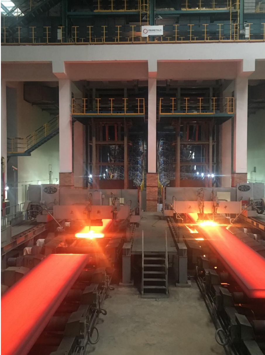
Two-strand continuous slab caster from Primetals Technologies at the Chinese steel producer, Shandong Iron & Steel Group Rizhao Co. Ltd.
