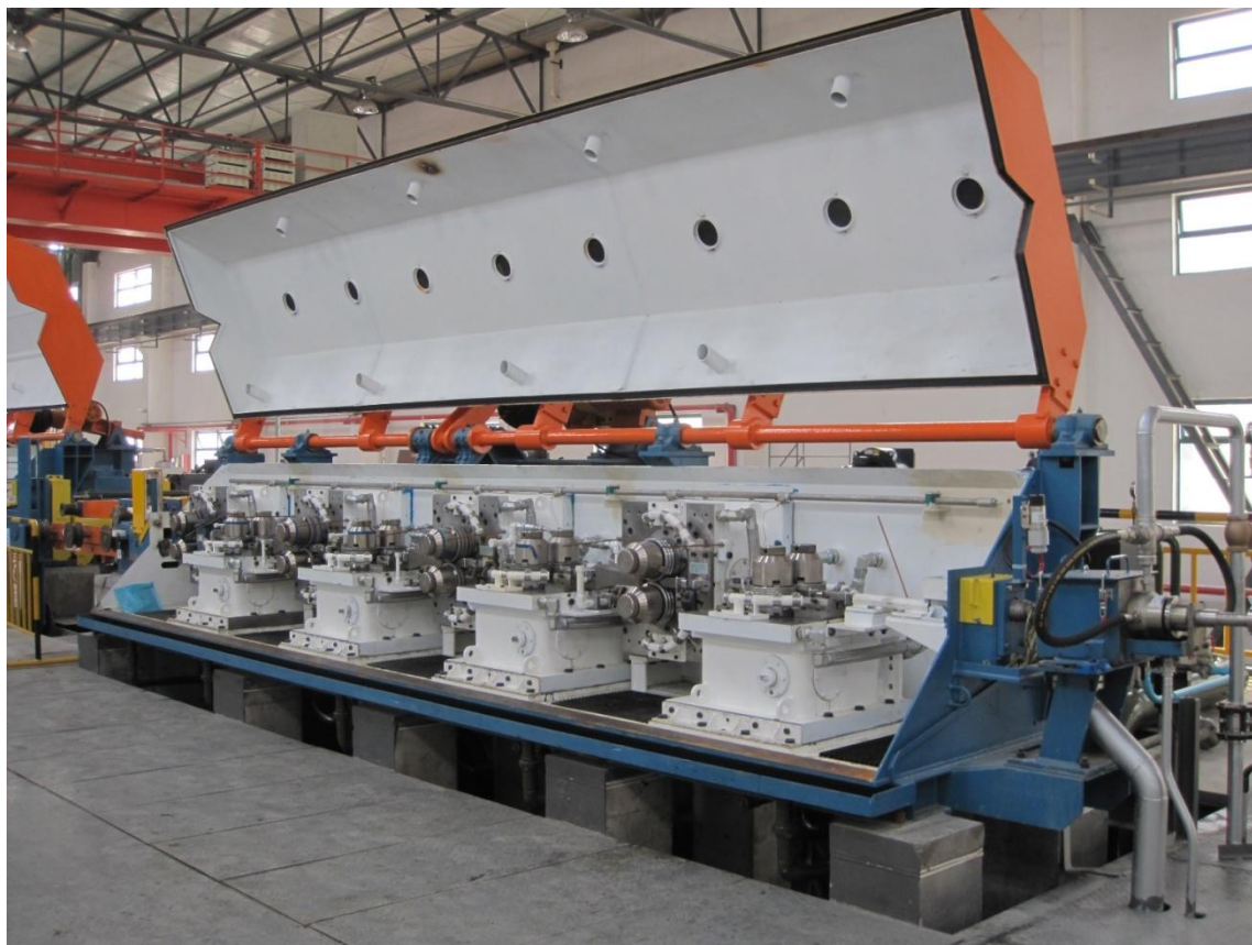
An SCR-7000 copper rod mill.
