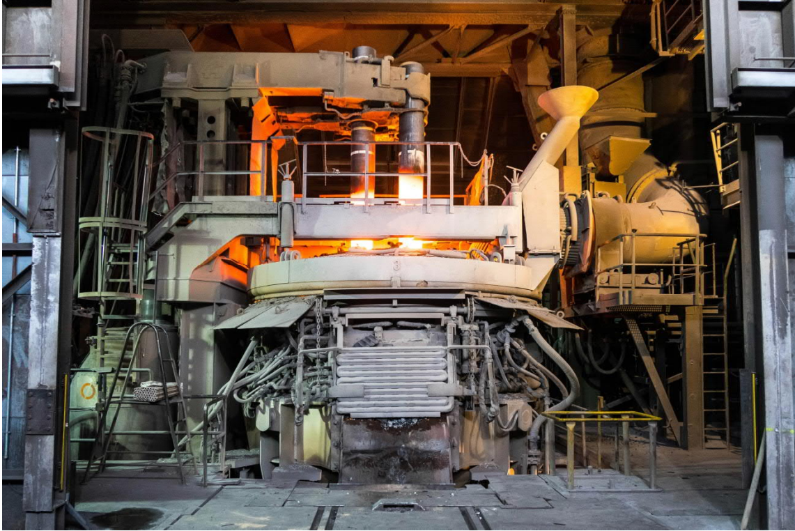
Electric arc furnace modernized by Primetals Technologies at BGH Edelstahlwerke GmbH in Freital, Germany
