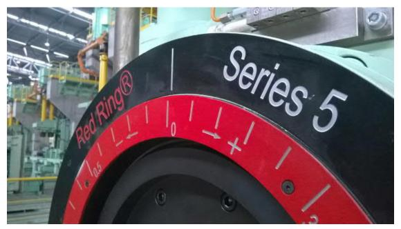
Red Ring generation 5 rolling stand from Primetals Technologies. The modernized rebar mill of Kamran Steel in Lahore, Pakistan will be equipped with a total of 14 stands.
