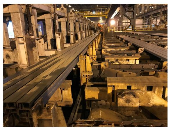
Stacking station for sections from Primetals Technologies
