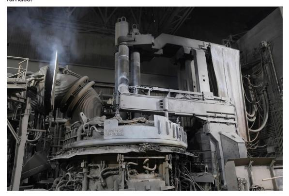
Electric arc furnace operated by Gerdau Special Steel North America at the company's electric steel plant in Monroe, Michigan, USA. Primetals Technologies will modernize the electric arc furnace and supply a new twin ladle furnace and new material handling system (photo: Gerdau Special Steel North America).
