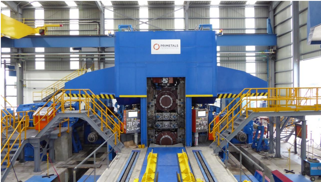
4-high reversing cold mill at TA 2000, S.A. de C.V.(Tyasa), Mexico
