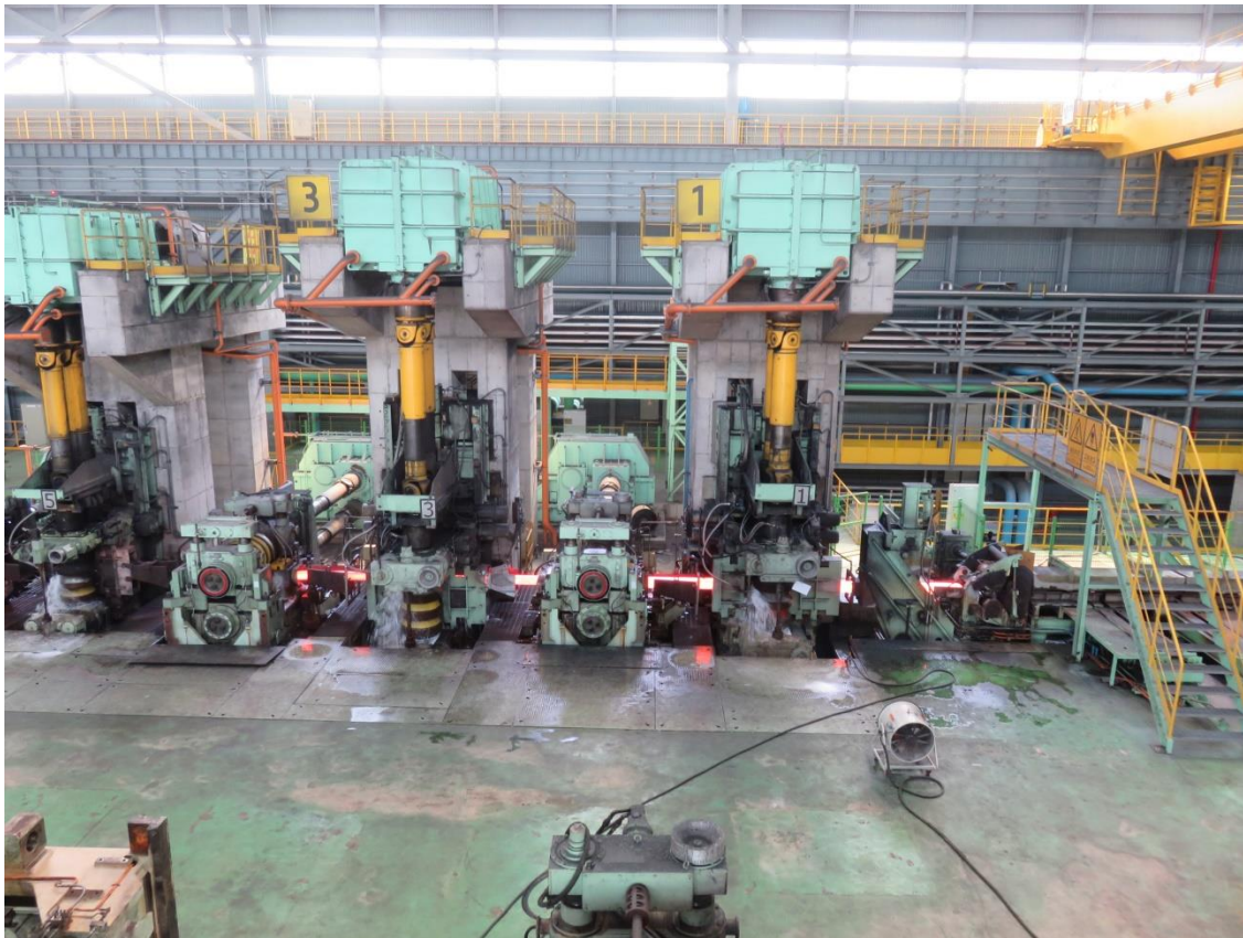
Small bar and wire rod mill from Primetals Technologies at Hyundai Steel in Dangjin, Korea
