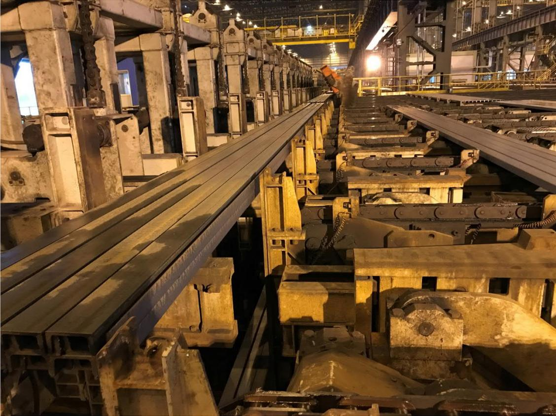
Stacking station for sections from Primetals Technologies
