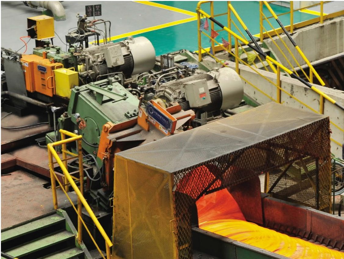
A Morgan Intelligent Pinch Roll and Morgan High-Speed Laying Head from Primetals Technologies
