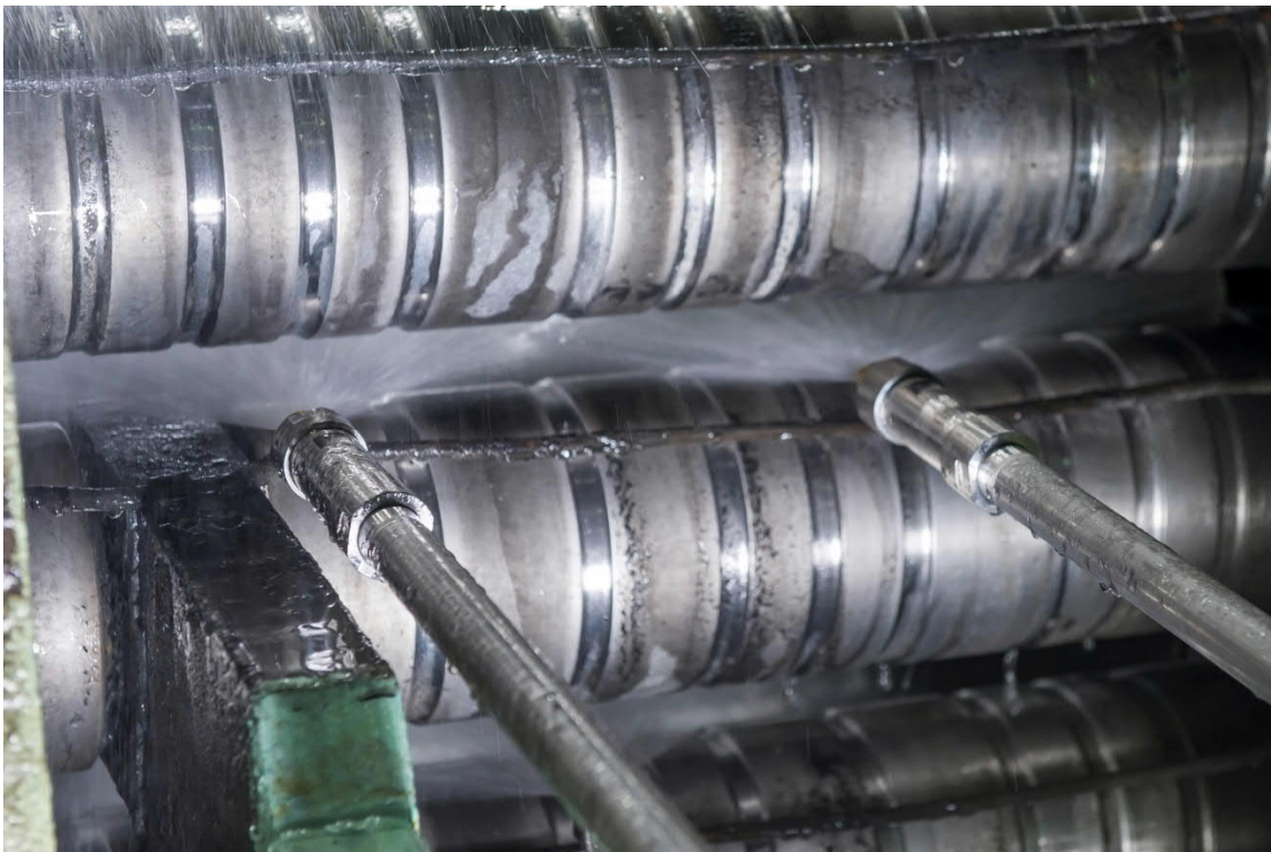
DynaJet Flex pulse-width cooling system from Primetals Technologies mounted in bender zone
