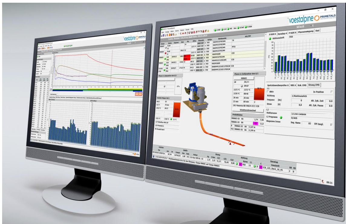
HMI interfaces of the new level 2 system supplied by Primetals Technologies for the CC8 continuous slab caster of voestalpine Stahl GmbH in Linz, Austria (Photo: © iStock.com/Eraxion)
