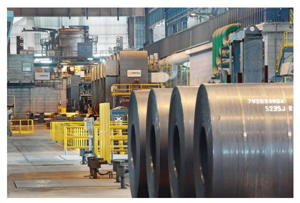
Arvedi Endless Strip Production directly linking casting and rolling in a compact layout
