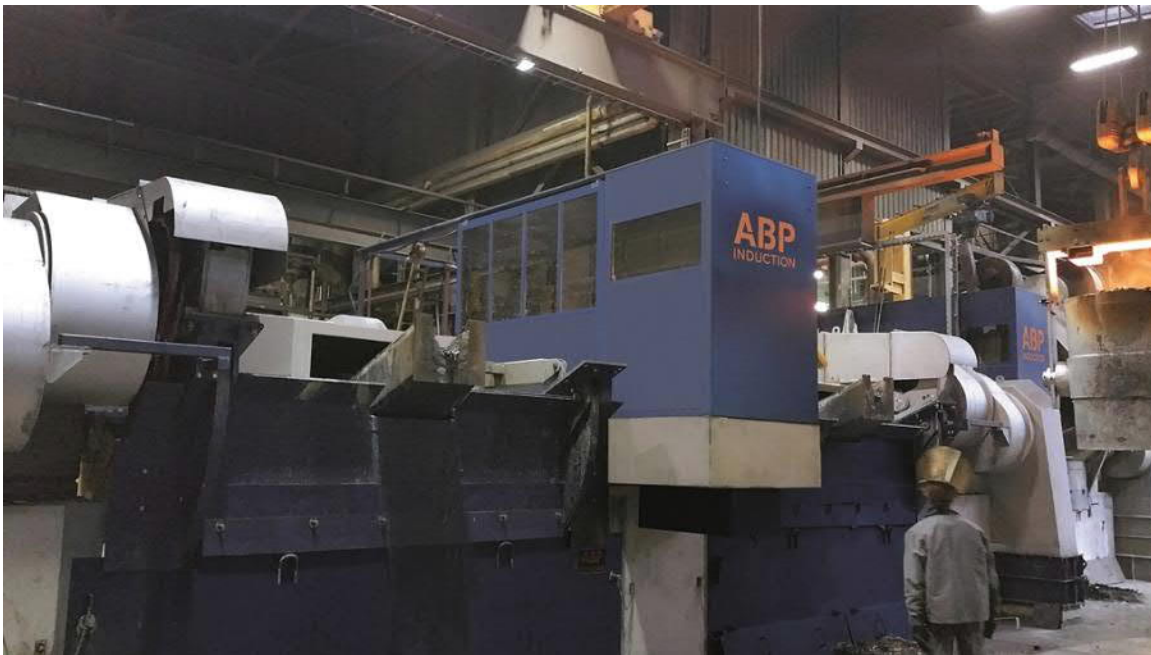
IFM 7 Twin Power from ABP, capacity 13.4 tons, rated power 6MW (Image courtesy ABP)
