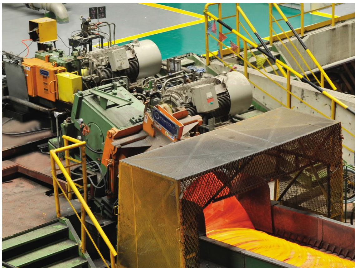
Morgan High Speed Laying Head and Morgan Stelmor cooling conveyor in a wire rod outlet.
