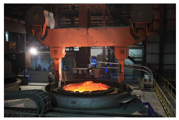
In the Dilovası meltshop of Turkish steelmaker Çolakoğlu Metalurji A.S. (Çolakoğlu), Primetals Technologies will upgrade an existing VD(Vacuum Degassing) plant to a VOD (Vacuum Oxygen Decarburization) plant.
