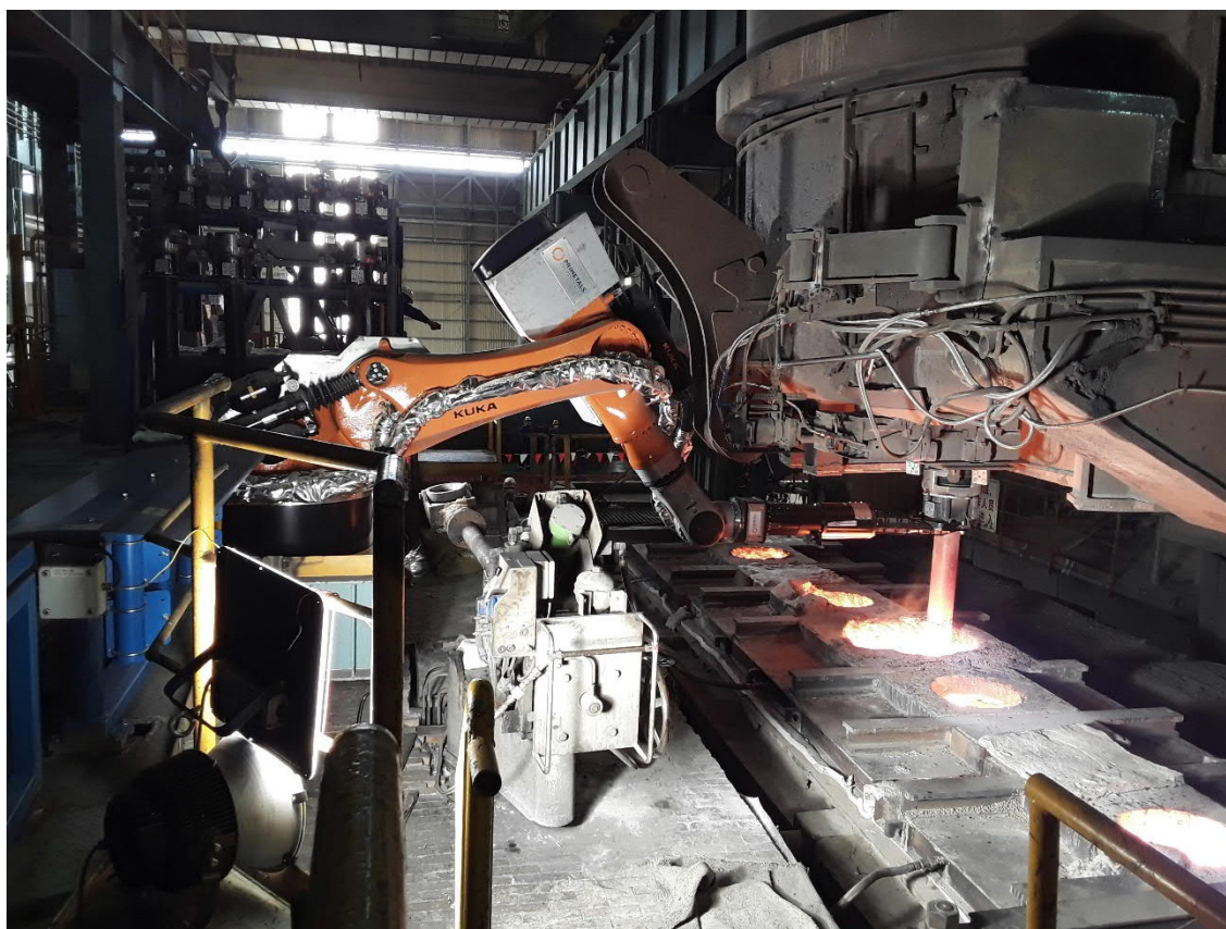
LiquiRob at Baosteel Meishan's CCM4 detaching a shroud
