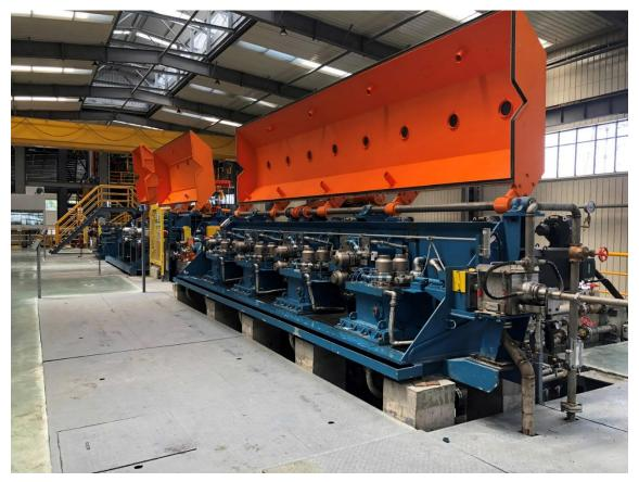
New SCR 9000 copper rod mill produced by Primetals Technologies, highest capacity ever supplied to Southwire Company LLC, for operation by Jiangxi Copper Company.
