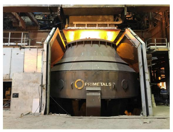
LD (BOF) converter modernized by Primetals Technologies at the steel works of the Chelyabinsk Metallurgical Plant (ChMK), part of the Mechel group in Chelyabinsk, Russia
