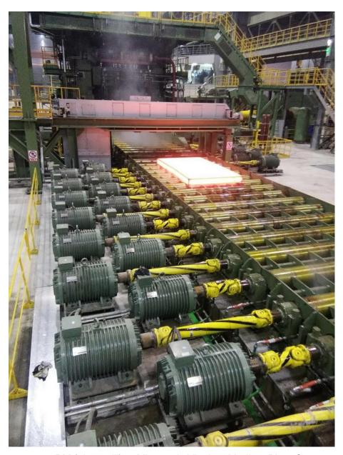
3800mm PM (plate mill) at Minmetals Yingkou Medium Plate Co., Ltd. in China. Primetals Technologies was responsible for the engineering, supply and commissioning of the L1 and L2 automation systems.
