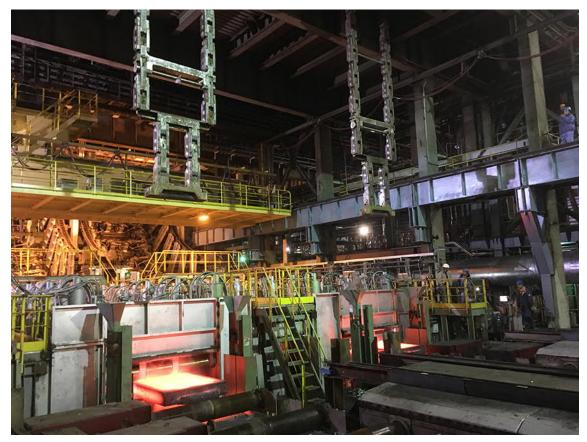
With the new fully automatic dummy bar top feeding system from Primetals Technologies, Baosteel can now start complete sequences as e.g. the takeover from hoist to car by pushing just one button.
