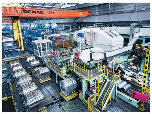
Four-high cold rolling stand at the AMAG rolling GmbH plant in Ranshofen, Austria. The plant is being modernized by Primetals Technologies. (Image courtesy AMAG rolling GmbH).
