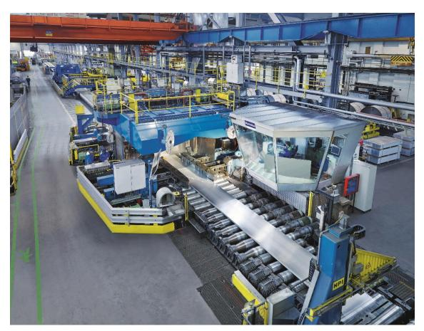
Two-high hot rolling stand at the AMAG rolling GmbH plant in Ranshofen, Austria. Primetals Technologies will equip the line with new converter equipment. (Photo: AMAG rolling GmbH)
