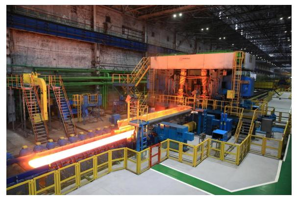
1,700 mm hot strip mill (HSM 1700) of Ilyich Steel in Ukraine. The hot strip mill was revamped by Primetals Technologies (Photo courtesy Metinvest).
