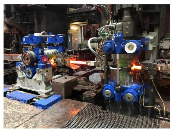
New Red Ring Series 5 stands by Primetals Technologies in the intermediate train of the long rolling mill of Stahlwerk Annahütte Max Aicher GmbH & Co. KG in Ainring-Hammerau, Bavaria, Germany
