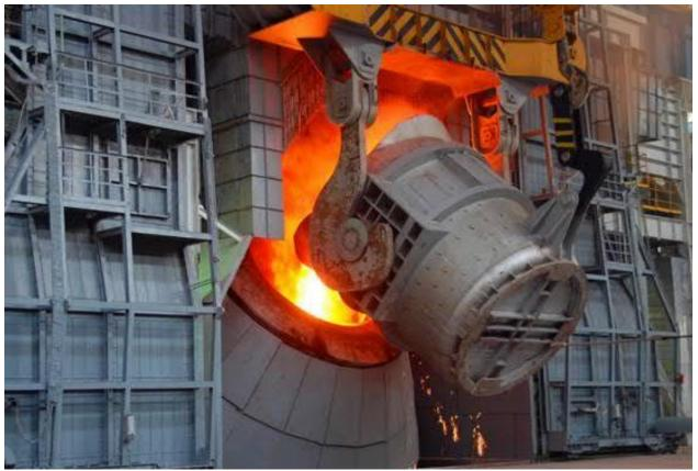
Primetals Technologies will upgrade existing BOF converter of Handan Iron and Steel to a KOBM converter including the complete automation system.
