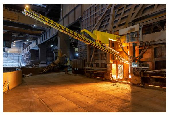
Semi-automatic horizontal temperature and sample-taking manipulator systems installed at the converter steel plant of Dillinger Hütte in Germany by Primetals Technologies (Image courtesy Dillinger Hütte)
