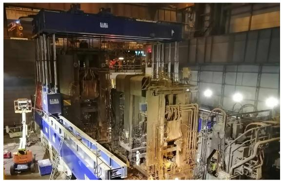
A special crane moves the rolling stand R1 to its new position as R 3 in the Arvedi ESP line of Acciaieria Arvedi in Cremona, Italy. The modernization project was carried out by Primetals Technologies and is part of an upgrade aimed at raising the line's production capacity to 3 million metric tons per year.
