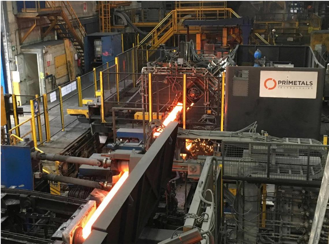
The ERT-EBROS billet welding system from Primetals Technologies installed at Ferriera Valsabbia S.p.A. in Odolo, Italy.
