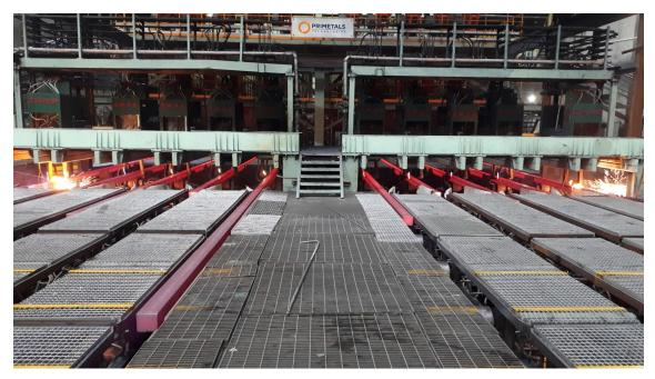
10-strand billet caster at the Changzhou converter steelmaking plant #3 of Chinese steel producer Zenith Steel. The caster was supplied by Primetals Technologies and is equipped with SRD segments for hard reduction and special technological packages.
