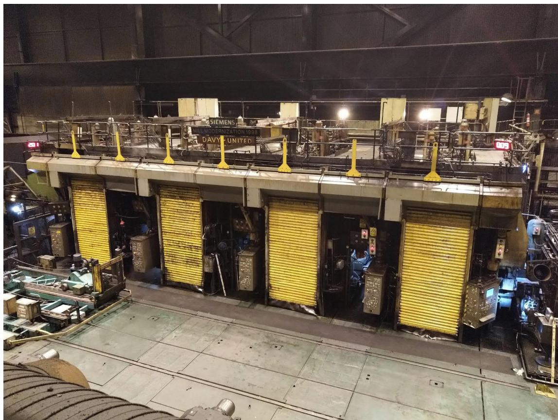
Tandem cold rolling mill in SSAB Hämeenlinna, Finland. The rolling mill is to receive new process automation from Primetals Technologies (Image: courtesy SSAB).
