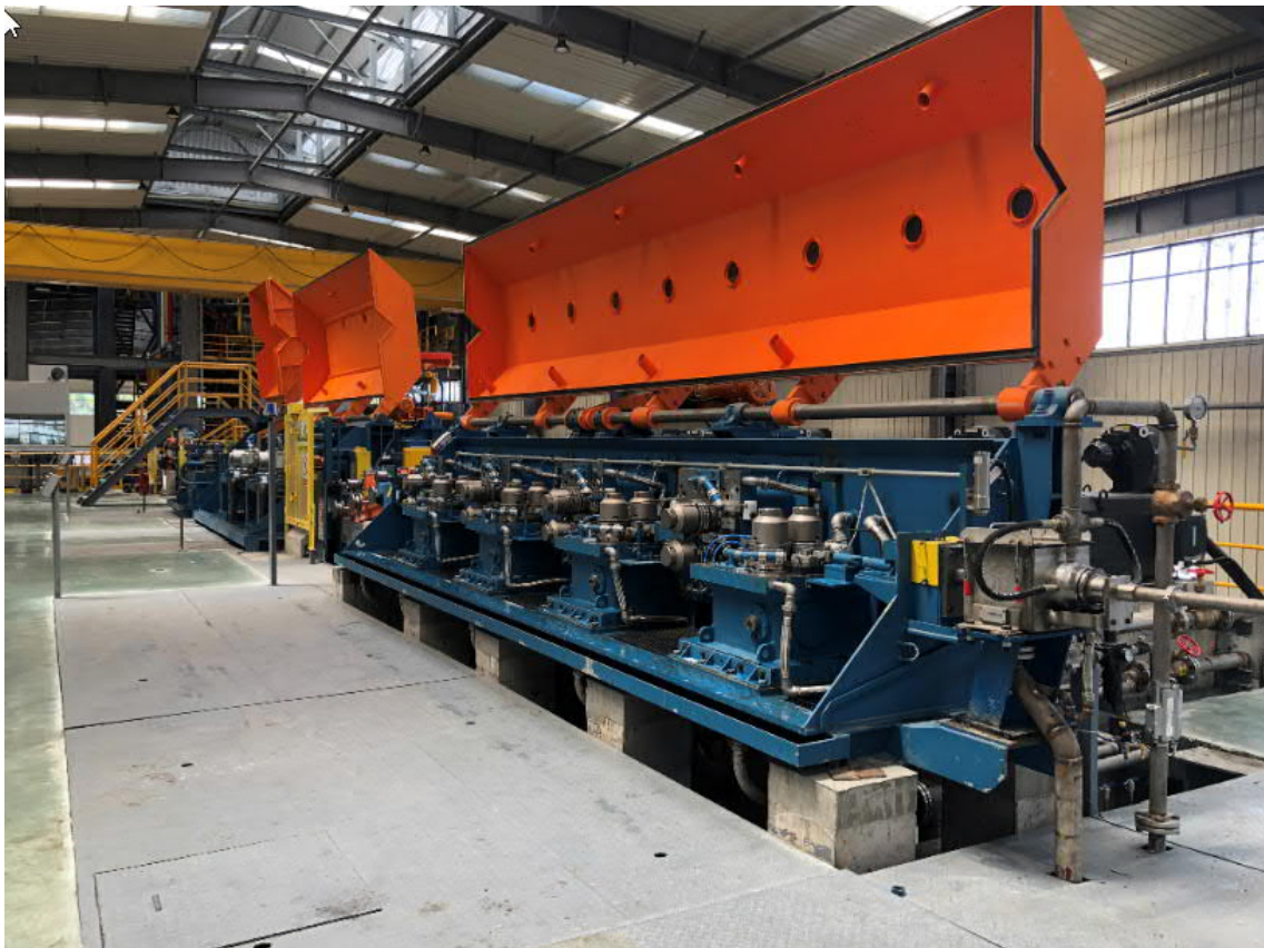
Standard Mill Arrangement for SCR 9000S copper rod mill produced by Primetals Technologies for Southwire Company, LLC
