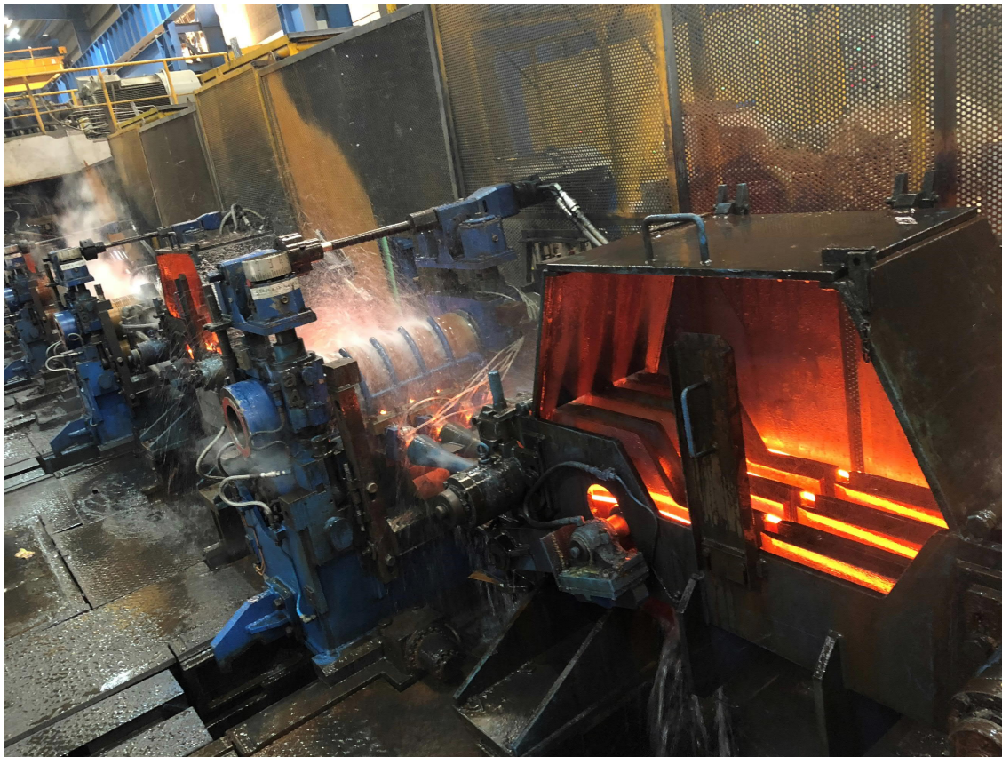
Four-slit rolling at the new bar mill of Amreli Steels Ltd., Pakistan, supplied by Primetals Technologies.
