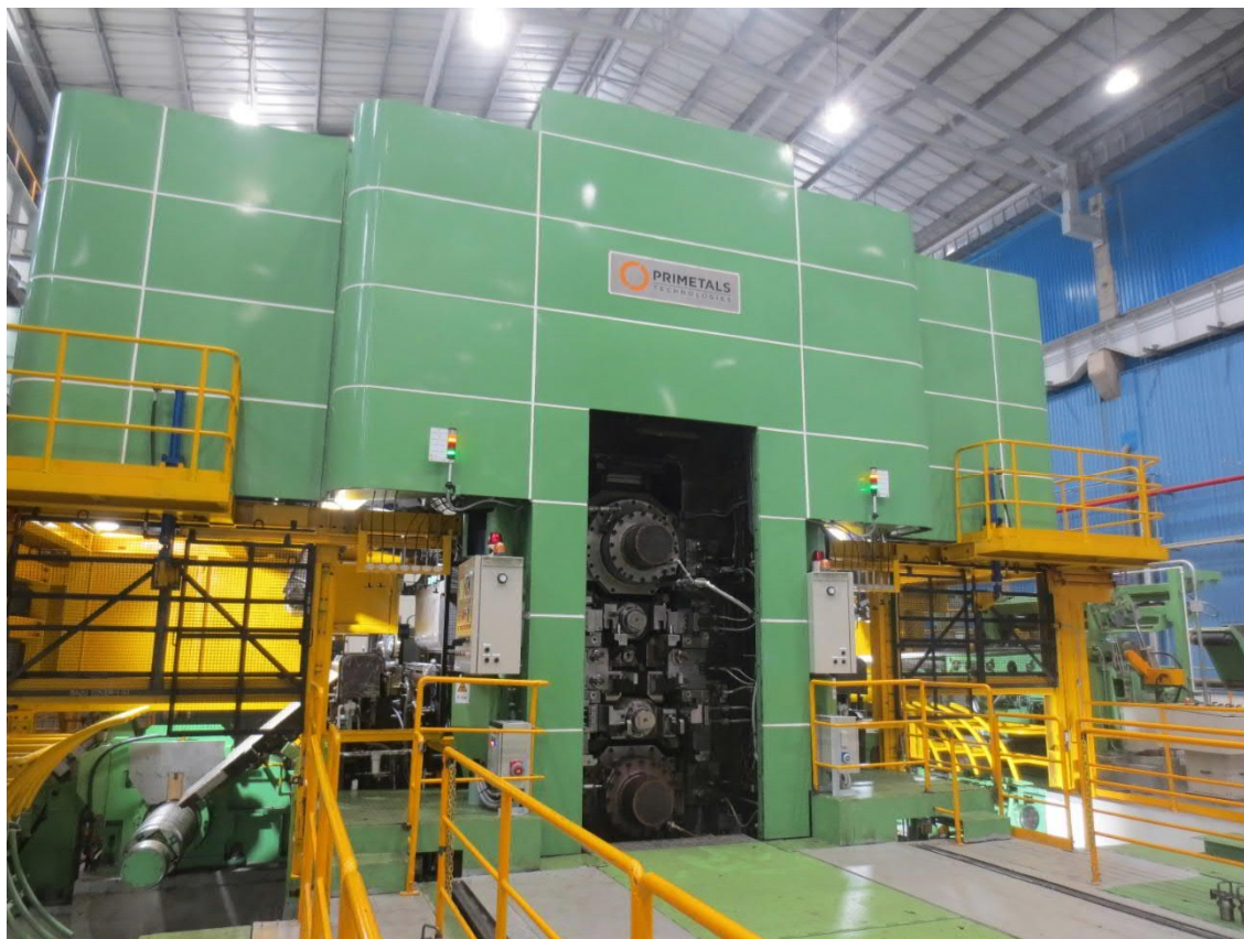
Primetals Technologies' first Hyper UC mill for lightweight construction materials in Vietnam
