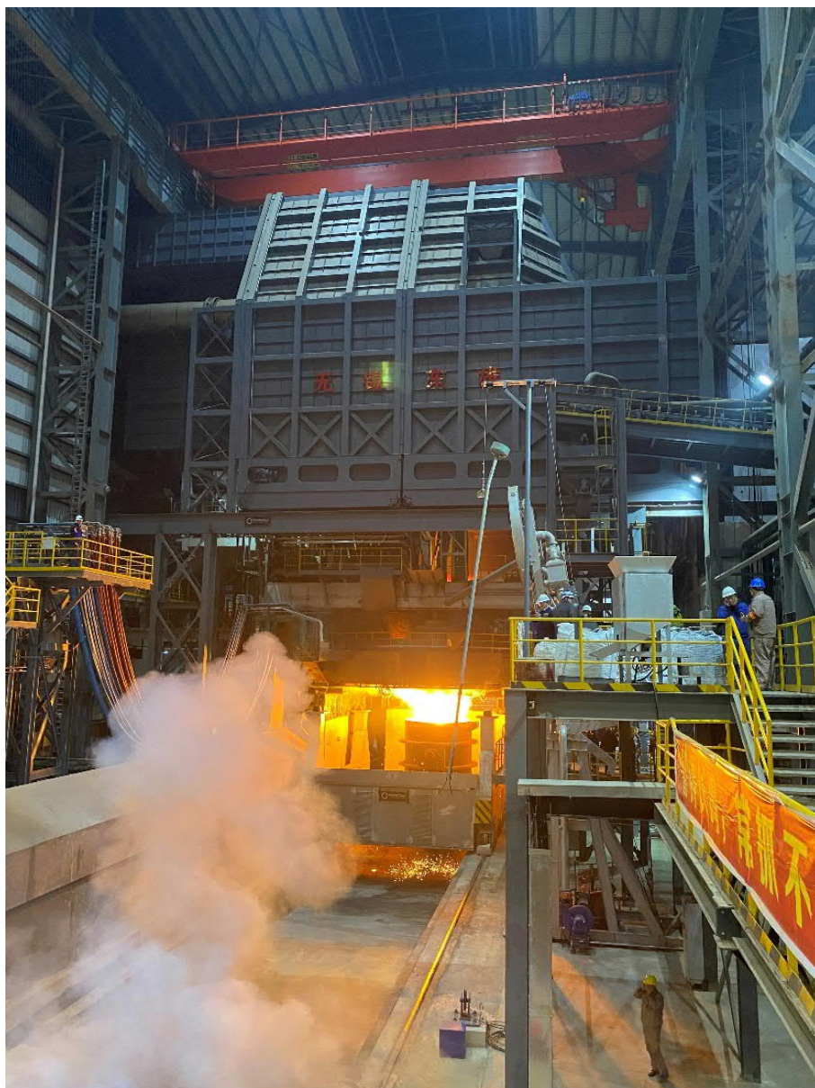
EAF Quantum with doghouse for highest environmental standards at Guilin Pinggang, China
